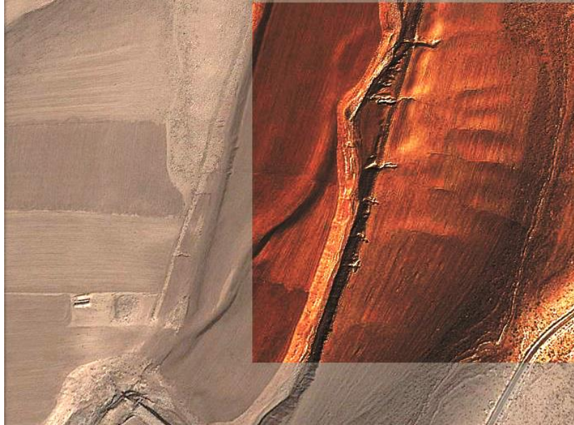
Fig. 3. Damages on the dike made by rainfall (Google Earth™ 2012).
